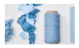
The project 'the ultimate recycled knitting yarn' aims to optimize the properties of sustainable knitting yarn, with a specific focus on reducing twist to minimize spirality issues in knits. Various yarn blends will be explored with the goal of creating the ultimate recycled knitting yarn. This will involve mechanically recycled fibers from Wolkat, where old clothing serves as a source for new clothing (fiber-to-fiber recycling).
