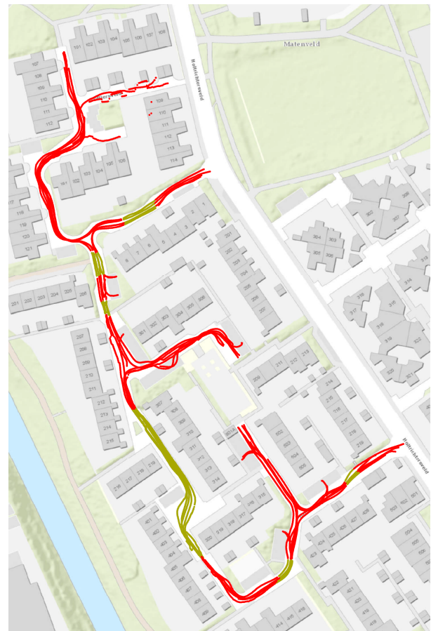
FIGURE 3. Applied pavement materials (red = concrete pavers, green = concrete paving slabs).
