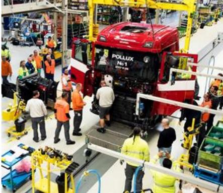
Scania Productions Zwolle ([www.scania.nl](http://www.scania.nl)) is a lean manufacturer which produces trucks, assembling on average 200 trucks per day, each configured to customer requirements. This requires strict control over production, whereby coordination between people and machines is crucial. The uptime is currently 97% which means that 3% of the time no production can take place. The goal of Scania is to increase uptime.
