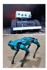
The research group recently created a proof-of-concept of a thermal SLAM algorithm operating during a fire incident. The system is capable of providing a sparse 3D-reconstruction, containing sufficient detail to plan movements and avoid obstacles. Some tasks such as crime scene or post-fire investigations however, require more refined knowledge of the environment.
