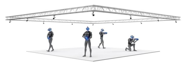
Optitrack lab with camera that can determine the position of optical trackers.
